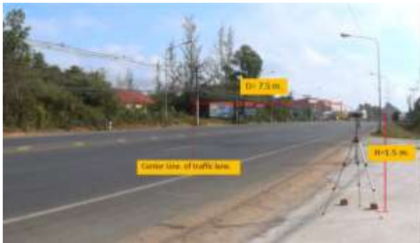
Fig. 6: Position and height of installed noise meter
