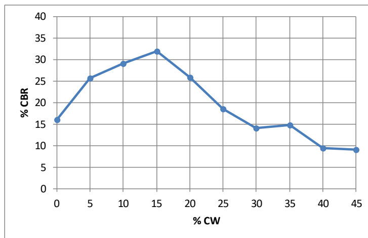
Figure 1 CBR value of soil sample mixed with recycle concrete
