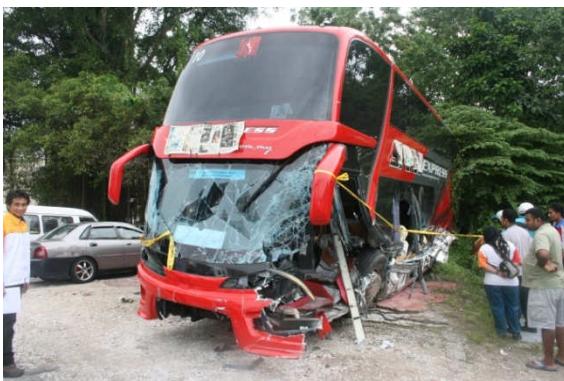
Figure 7 Severe damage on the nearside of the bus due to collision with bridge parapet
