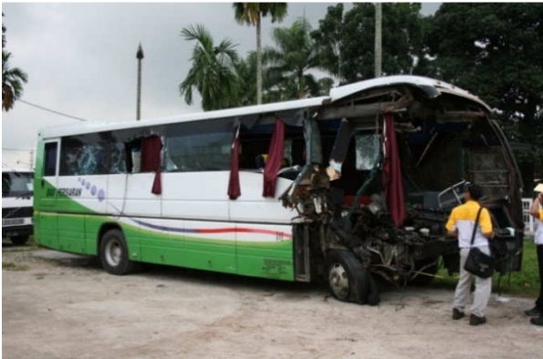
Figure 8 Condition of the damaged bus with brake failure
