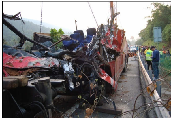
Figure 4 Detached roof as a result of rollover crash
