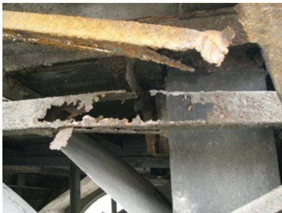
Figure 5 Severe corrosion on bus structure
