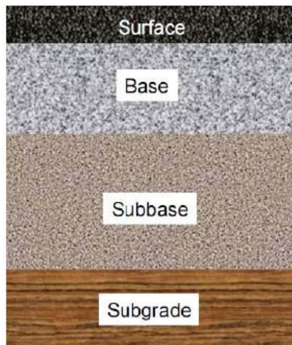
Figure 1. Basic components of a typical pavement system
