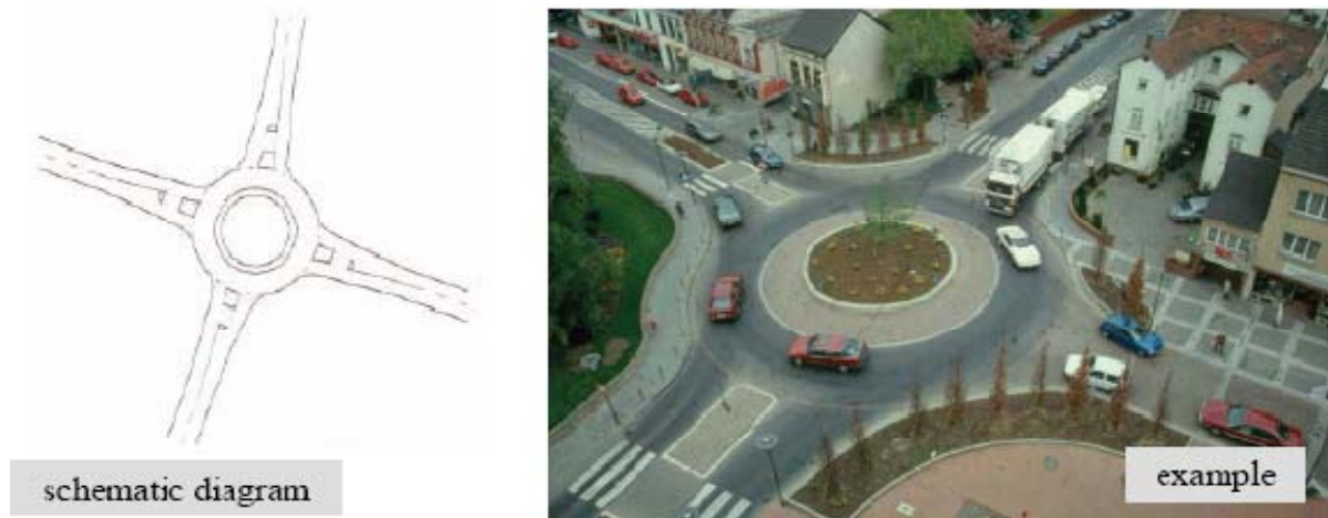
Figure 10. Compact one-lane roundabout inside built-up area, mirrored figures (FGSV, 2006, Brilon, 2005)
